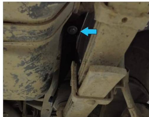
4. Install the rear left mounting bracket (pos.6) using factory bolts (Fig.4).
