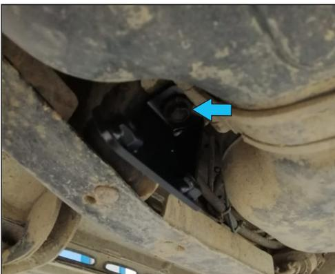
3. Install the front left mounting bracket (pos.4) using factory bolts (Fig.3).
