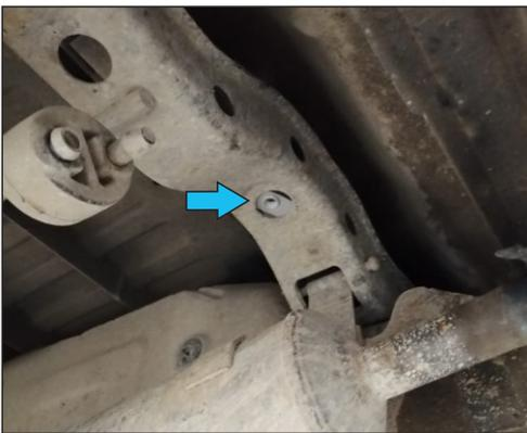
1. Place Insert Nut M10x65 (pos.G) in frame rail (Fig.1).
