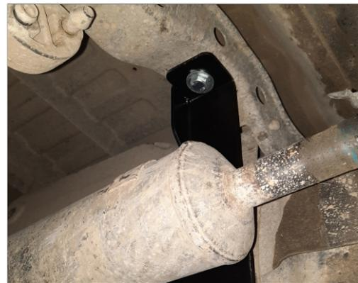
2. Install the front right mounting bracket (pos.3), using Bolt M10x25 (C), Flat washer 10 mm (pos.E) (Fig. 2).
